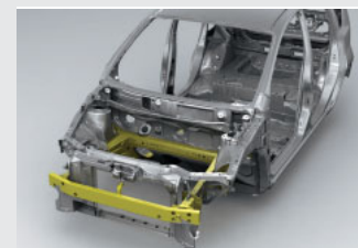
A crash-compatible Zone Body construction (Note)
