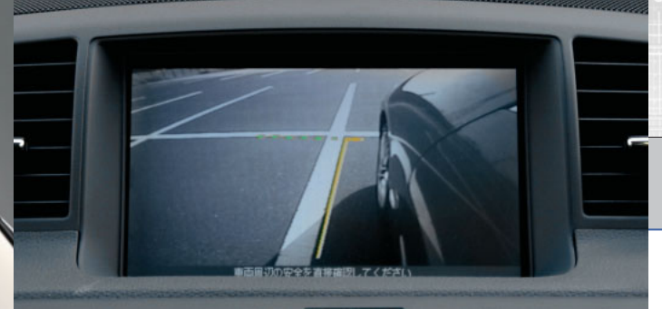
Side Blind Monitor — a highly sensitive infrared CCD camera is used to display the left front-side of the vehicle on a monitor at night to reduce blind spots (Fuga)
