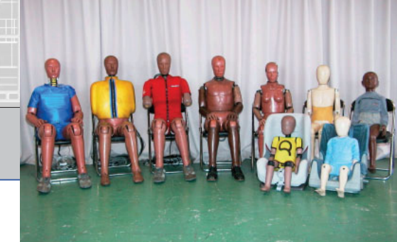
Specially designed dummies are used to confirm the safety performances of vehicles
