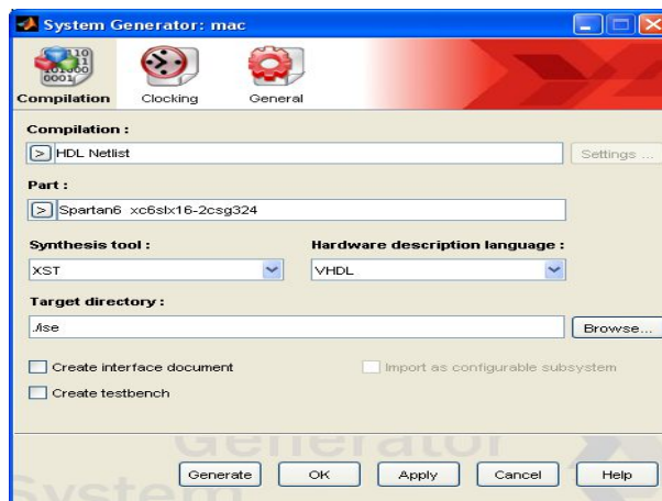
Figure 18: System Generator Parameters for Generating VHDL Code
