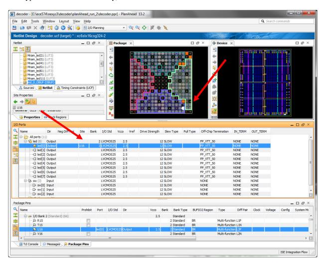
With reference to the Nexys3 Reference Manual complete the pin information for the rest of the led and sw ports.
