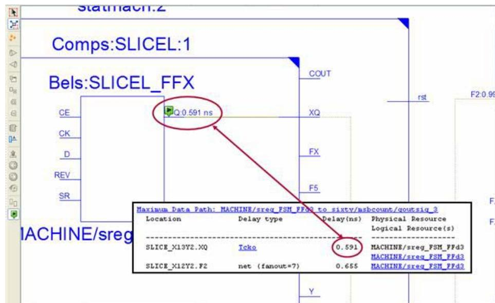
Figure 6-10: Data Path Annotated with Timing Delays
