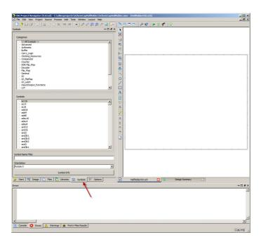
Select **Logic** from this list and a list of simple logic gates will be shown in the lower **Symbols** scroll box. For the half adder, we will require a 2 input XOR gate and a 2 input AND gate. To add a simple logic gate to the circuit, left-click to select a symbol from the Symbols list, drag the cursor to the pallet where you want the symbol to be placed, and left-click again to drop the gate in the schematic. You can also find a symbol by typing a name into the symbol name filter.
