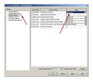
Highlight startup options and change the switch name "-g StartUpClk" value to JTAG clock. Press Apply then OK.
