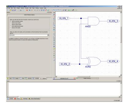
9. Go back to regular cursor mode (Select Mode Icon) And double left-click on an I/O marker. When the I/O marker's object properties dialog box appears, select the Nets category and enter a meaningful value for the Name field of the I/O marker. The finished dialog box should look similar to the following:
