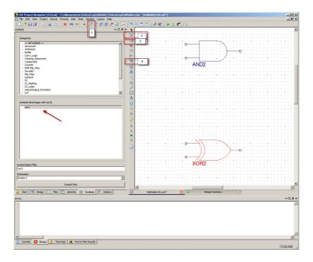
The figure above highlights the tools necessary for creating a basic digital circuit using schematic capture:
