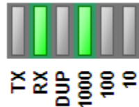
Ethernet status LEDs
