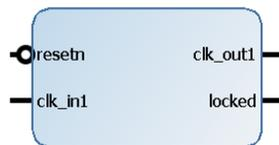
Figure 8: Clocking Wizard block with active-low reset and single-ended clock input.
